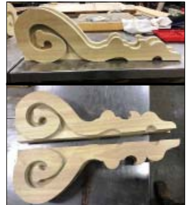
The completed corbels.
