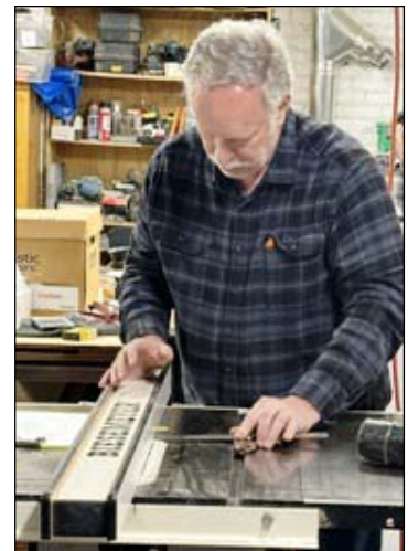
Checking fence alignment.
