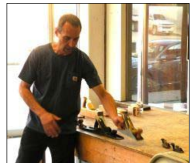
Showing the differences between jointer and jack planes.
