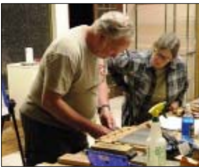
Showing how to set up the sharpening jig.
