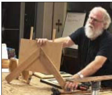
Showing the jig to cut 45° frame corners.
