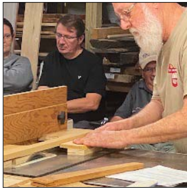
Cutting a part using the L-fence.
