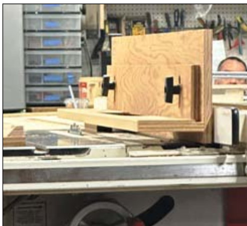
The L-fence attached to the table saw fence.
